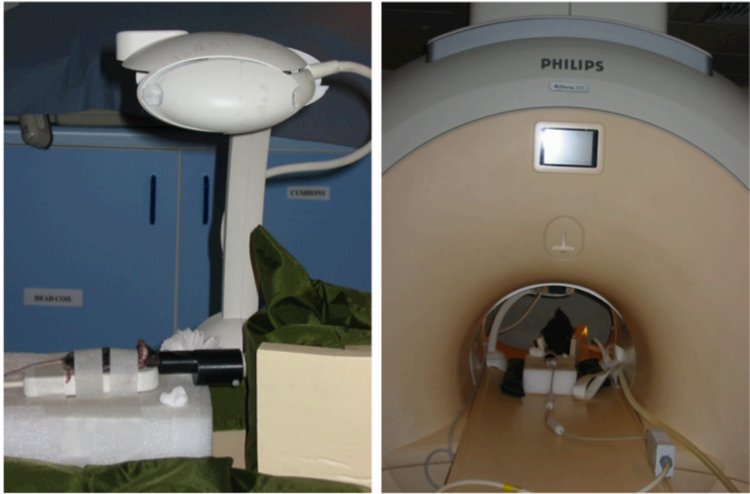
Figure 1.7- Set-up of 3T scanner for pre-clinical applications
