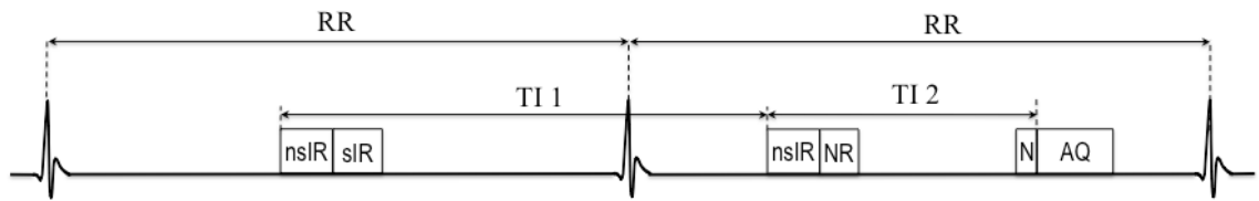
Figure 6.4- TIR4ASL sequence in 2 RR intervals, which increases the labelling time ( TI_1 + TI_2 ) and allows for venography. nsIR: Adiabatic non-selective inversion pulse. sIR: Selective inversion pulse, NR: Navigator restore pulse. N: Navigator, AQ: Image acquisition.
